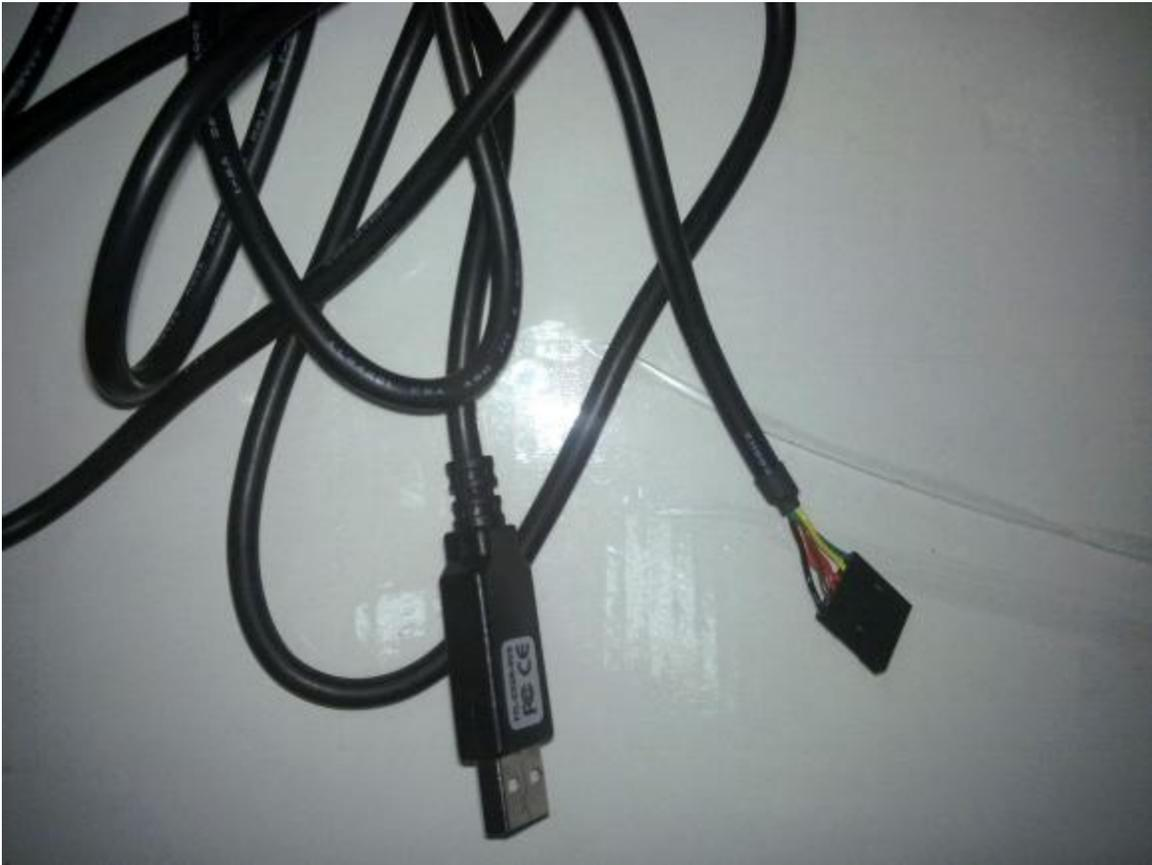
As all pins on the serial end of the cable are not useful ( We need only three pins) we need to open the serial end of the cable and separate three pins that are useful to us from the rest of the pins.
